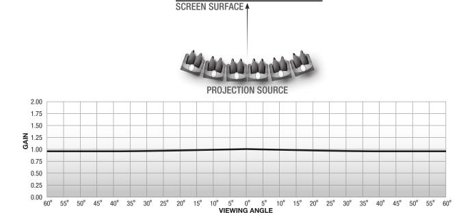
GAIN I.0 VIEWING ANGLE 180° THICKNESS 0.42 MM FULL HD COMPLIANT
