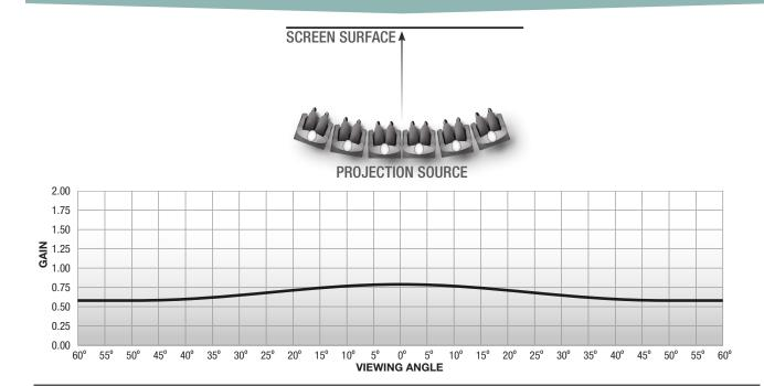
GAIN 0.8 VIEWING ANGLE 180° THICKNESS 0.37 MM 8K COMPLIANT
