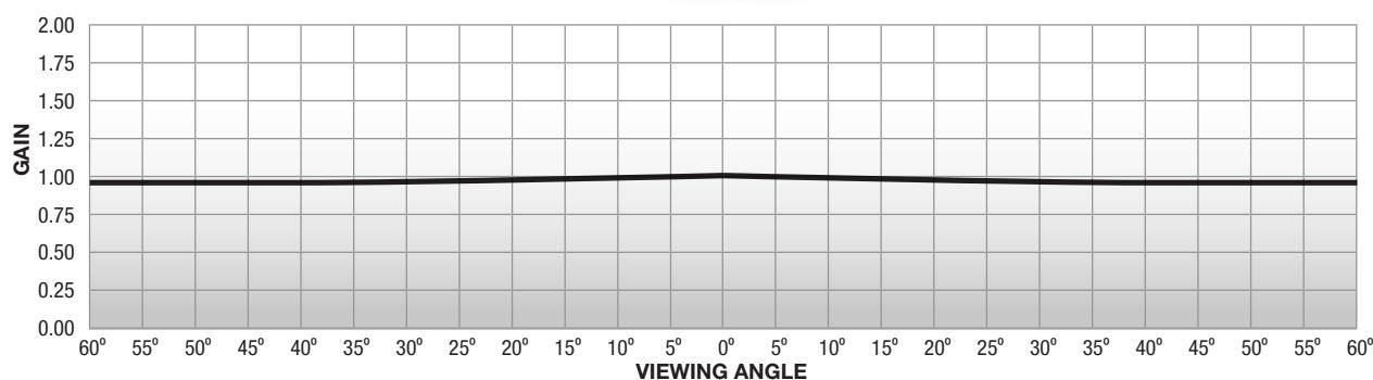
**GAIN 1.0   VIEWING ANGLE 180°   THICKNESS 0.5 MM   FULL HD COMPLIANT**
